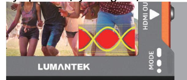
ez-SHV+ is useful for checking the input SDI cable's quality as a simple measurement tool through the displaying of eye-pattern. If the eye-pattern shows thick, then it means input video signal quality is poor.
