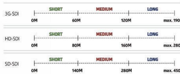
ez-SHV+ detects cable length automatically up to 190 m at 3G-SDI. Cable length will be shown as 'SHORT', 'MEDIUM' and 'LONG'.
