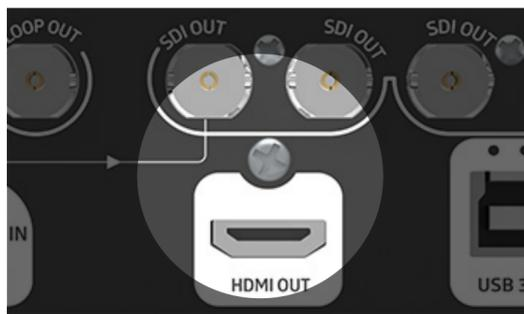
ez-DSK distributes the video into 1 Clean source and 5 CG'ed sources (4 SDI & 1 HDMI). You do not need an extra distributor or a converter for HDMI output.
