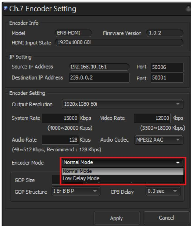
Set the delay mode between the Encoder input and output.
