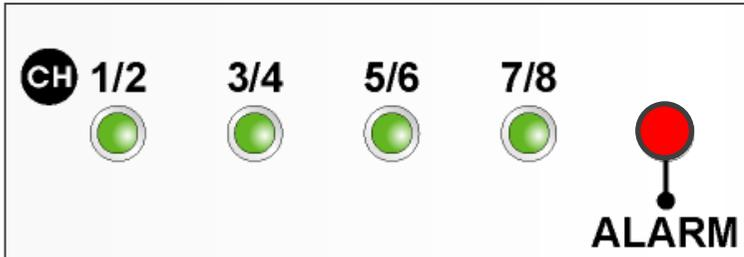
CH 1/2 LED - indicates LAN active Status of CH1 and CH2.
